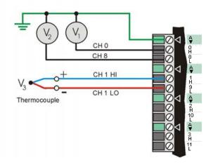
Figure 1. Single-ended voltage connections (V<sub>1</sub> and V<sub>2</sub>) and differential thermocouple connections (V<sub>3</sub>)
